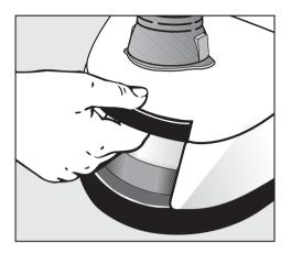
To remove the dustbag, hold the bag by the collar and pull it out of its holder.
